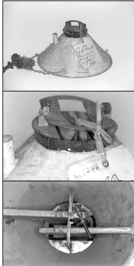
Figure 6. Patent model for John S. Tough's lamp, No. 1246 (1839). The screw underneath that moved a plate at the top up or down to control air flow, making it unnecessary to raise the wick or the glass shade, would have been mounted vertically, but has become dislodged. In the collection of the National Museum of American History.
