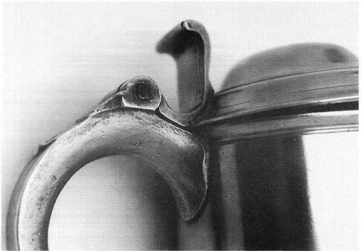
Figure 7. Close-up of detail of casting faults on handle. Note low profile of first dome on lid of tankard.
