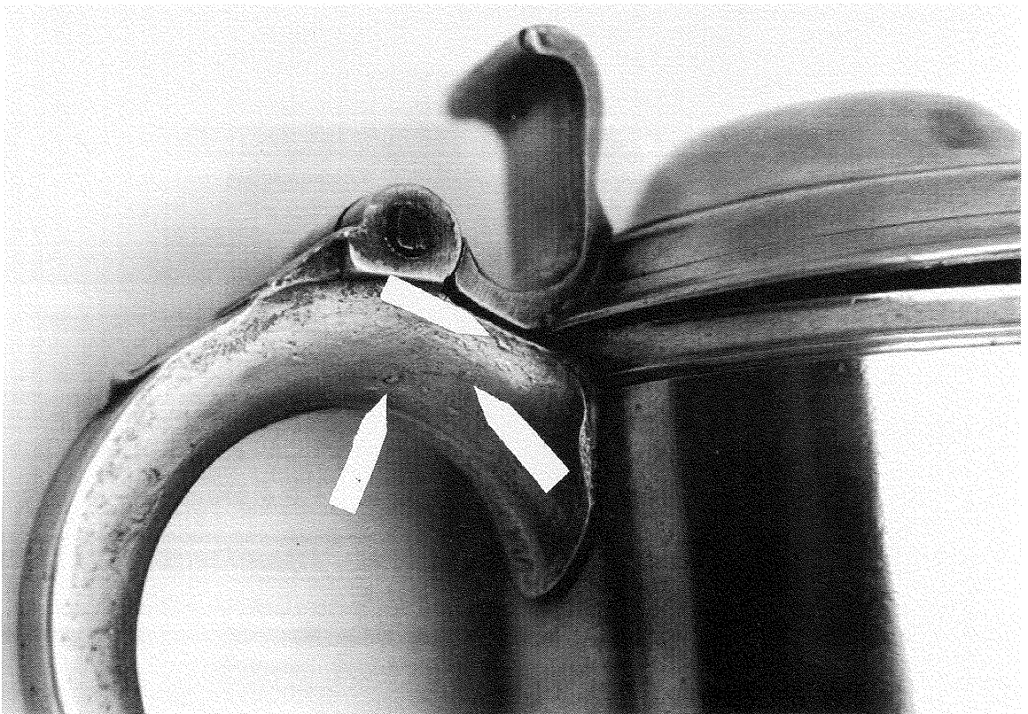
Figure 8. Same close-up with arrows pointing out small casting faults from mold (little bumps). The identical faults are present on all three tankard handles.
